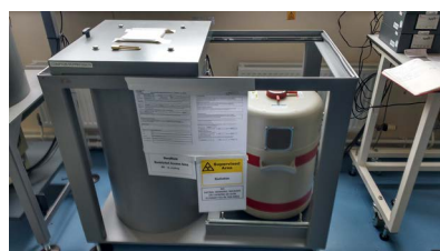
The high-sensitivity Broad Energy Germanium detector with Compton Suppression capability. The detector is hosted and managed at the Culham Centre for Fusion Energy, Abingdon
