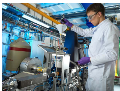
Callum Robinson, University of Manchester PhD student, demonstrating the loading of a sample containing uranium onto Diamond's I20-scanning beamline © Diamond Light Source
