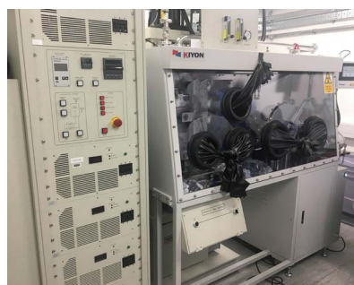
Spark Plasma Sintering Furnace with attached glovebox
