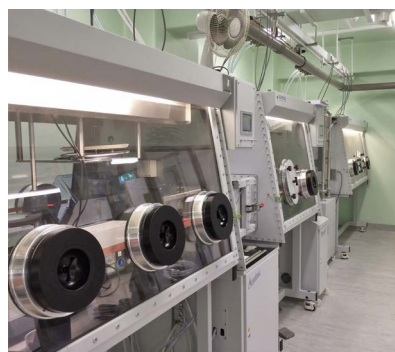
Uranium glovebox suite for sample production and preparation
