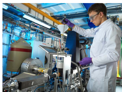
Callum Robinson, University of Manchester PhD student, demonstrating the loading of a sample containing uranium onto Diamond's I20-scanning beamline © Diamond Light Source
