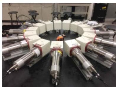
15 of the 32 liquid scintillation neutron assay system hosted and managed at Lancaster University. The image was taken during work at the Oak Ridge National Laboratory, USA, using a selection of their high-activity sources to measure neutron multiplicity
