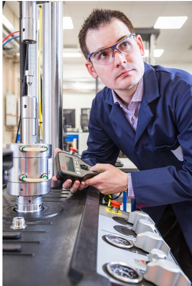
Set-up of a servo-hydraulic fatigue test station
